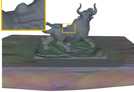
Figure 6. Visualization of norms of weighted feature vectors, \mathbf{F} \cdot \text{diag}(\mathbf{w}) . The norms of low-, middle-, and high-frequency features are visualized as red, green, and blue channels, respectively.
