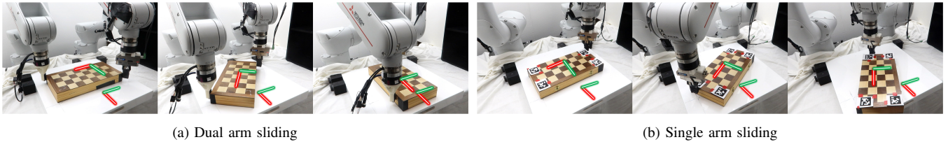
Fig. 7: Demonstration of sliding manipulation of a box in hardware experiments using the proposed algorithm. In Fig. 7a, the robots do not change the contact location on the object. In Fig. 7b, the robot has to change its contact location to accomplish its task. The arrows represent the current orientation of the object and its desired orientation at the terminal time-step. The Apriltag system is used for feedback during the change of the contact location to ensure that the robot makes contact in the correct location.
