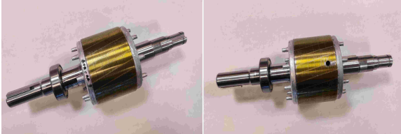
(b) The left figure shows a healthy rotor and the right figure shows a broken-bar rotor.
