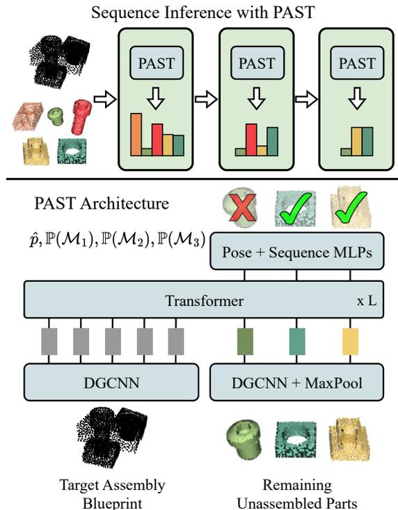
Fig. 2: Sequence inference pipeline and PAST architecture. (Top) PAST operates sequentially to estimate the assembly probability  $\mathbb{P}(\mathcal{M}_i)$  for each remaining part. The part with the highest probability is chosen for assembly. (Bottom) Using the third block as an example, PAST selects one part for assembly from the three remaining options. PAST also performs pose regression for each part  $\hat{p}$  as an auxiliary task.
