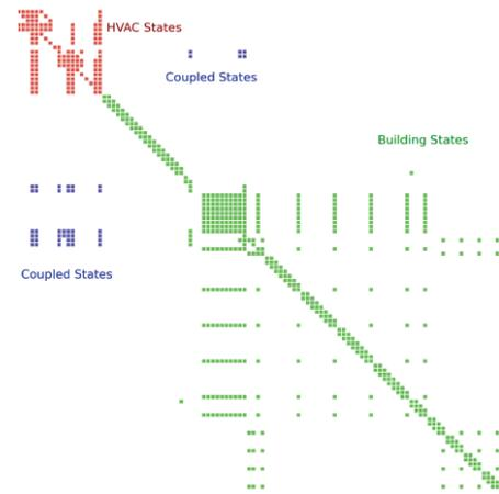
Figure 2: Jacobian sparsity pattern for a system model of a vapor compression cycle in a building (Chakrabarty et al., 2021).
