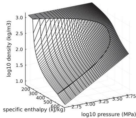
Figure 3: Density surface of refrigerant R32 as a function of pressure and specific enthalpy.
