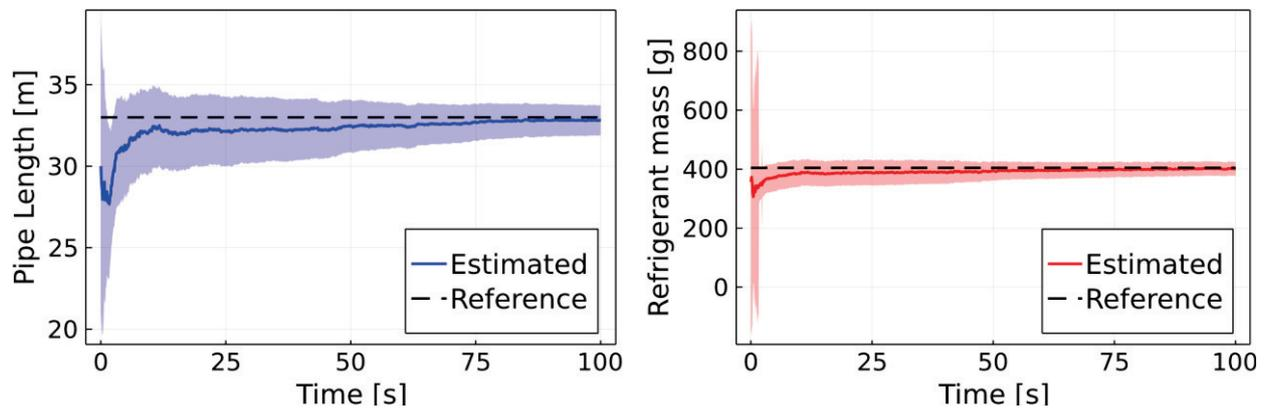
Figure 5: Solid lines show estimated pipe length (left) and refrigerant mass (right) while shaded areas show  $3\sigma$  bounds. Dashed lines show reference parameter values.
