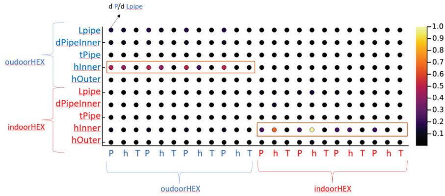
Figure 4: Local sensitivities of cycle states with respect to model parameters. Sensitivities are normalized and scaled between 0 and 1.
