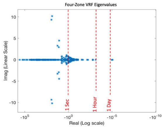
Figure 1: Eigenvalues of the Jacobian for a four-zone VRF system, with the real-axis on a logarithmic scale.
