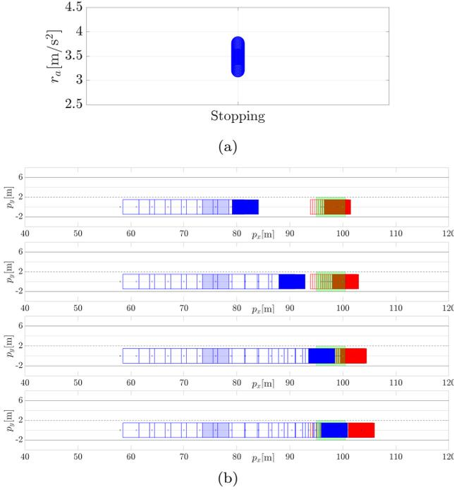
Fig. 3. Stopping scenario with 1 maneuver. (a) feasible values of commanded acceleration  $r_a$ . (b) execution of the maneuver with minimum  $r_a$ . Ego (blue) and other (red) vehicles: current (solid), past (border only), and at maneuver start (shaded) positions. Stop region (green). Snapshots after  $t = 0.5, 1.5, 2.5, 3.5$ s from maneuver start.
