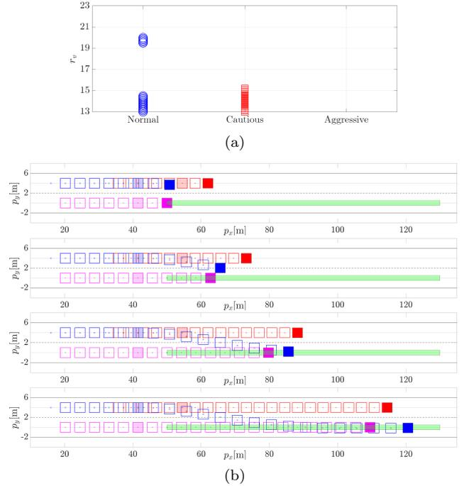
Fig. 2. Lane change scenario with 3 feasible maneuvers. (a) allowed values of commanded velocity  $r_v$  for each maneuver. (b) execution of the *normal* maneuver at maximum feasible  $r_v$ . Ego (blue) and other (red, purple) vehicles: current (solid), past (border only), and at maneuver start (shaded) positions. Region of lane change completion (green). Snapshots after  $t = 0.5, 1.25, 2.25, 4$ s from maneuver start.
