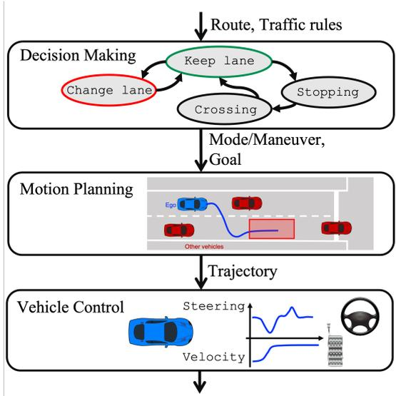
Fig. 1. Multi-layers automated driving system: current (green) and next (red) maneuver/mode in decision making, goal (red) and trajectory (blue) in motion planning, and control signals (blue) in vehicle control.
