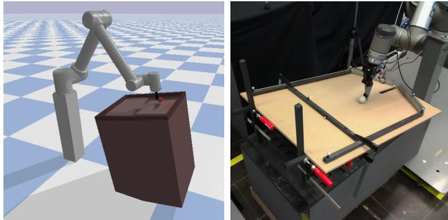
Fig. 1: Our *active exploration* strategy evaluated on a challenging *Tilted Pushing* task in simulation (left) and on the real robot (right). The agent needs to learn the dynamics of the task and identify a sparse reward model in order to bring the ball to a target location. The robot learns to solve the task online in the real setting from scratch.
