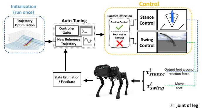
Fig. 1: **Auto-tuning framework.** We initialize the reference trajectory for the first few footsteps and CoM base using trajectory optimization. Then, auto-tuning is applied to estimate new reference trajectories which account for desired physical parameters. Further, auto-tuning is applied on cost function weights for a stance controller (MPC) and feedback gains of a swing controller (PD).
