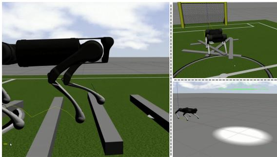
Fig. 4: **Results for robust locomotion on uneven terrain.** After auto-tuning the stance and swing controllers, we employ the robot on several test cases to demonstrate robust locomotion. We show the robot traversing over and on large beams and planks in the left and top right with a trot gait, respectively, and demonstrate a successful jumping gait in the bottom right. The robot is not aware of the obstacles and must overcome them by using the auto-tuned controllers.
