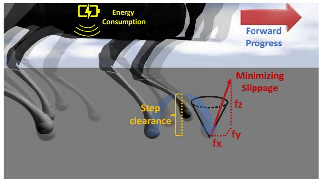
Fig. 2: **Auto-Tuning reference trajectories in Gazebo.** The robot follows a reference trajectory that is being tuned by the auto-tuning formulation. The figure shows the robot following a desired velocity (forward progress), a desired foot height (step clearance), minimizing foot slippage (ground reaction forces), and minimizing energy consumption.
