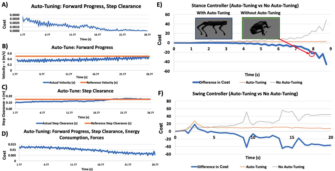
Fig. 3: **Auto-Tuning results.** The auto-tuning method successfully calibrated control parameters that generate reference trajectories (A-D), and controller gains (E-F). To make this evaluation, we used the cost as calculated using (2). The cost decreases (A and D) as the control parameters (e.g., forward progress and step clearance) get to their desired reference values. In E-F, we show the difference between the cost when not auto-tuning with the cost when auto-tuning.
