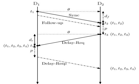
Fig. 2. Two-way packet exchange for synchronization. A filled circle dot denotes a timestamp in the event message recorded at its transmission and reception. The processing time taken at all the nodes is assumed to be  $p$ .
