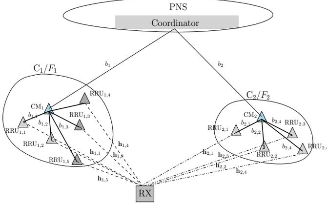
Fig. 1. Illustration of the proposed MC-dRRUS with five RRUs in Cluster 1,  $C_1$ , and four RRUs in Cluster 2,  $C_2$ . Two central nodes highlighted in each cluster are assigned as CMs to control the other RRUs in its cluster.
