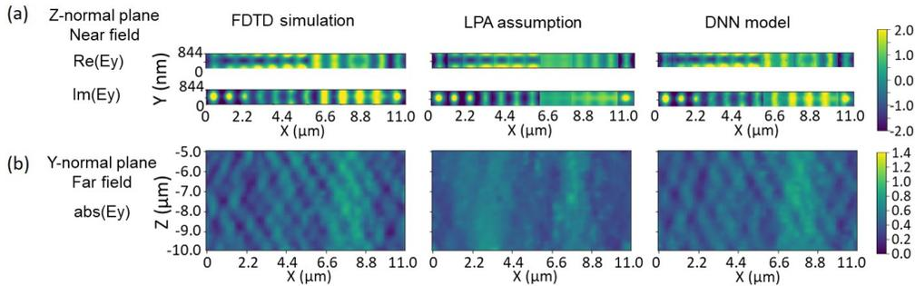
Fig. 3. (a) Z-normal plane near fields of  $E_y$  calculated by FDTD simulation, LPA and the DNN model on a 13-unit super cell. (b) Far field projection of  $E_y$  in Y-normal plane, obtained based on the near fields in (a). The DNN model improves the estimation accuracy in both near and far fields.
