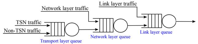
Fig. 1. The multi-level queue abstraction of the network stack of a TSN device. Periodic TSN packets generated at the application layer are buffered with aperiodic non-TSN packets in a transport layer queue. TSN packets have to traverse subsequent queues at lower layers until they are finally transmitted.
