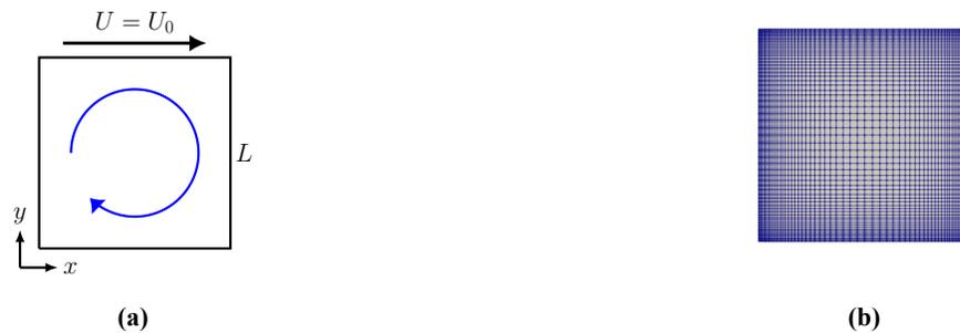
**Figure 4:** Illustration of the 2D cavity case: (a) Schematic (based on Figure 4-1 of Zuo (2010)) (b) Mesh
