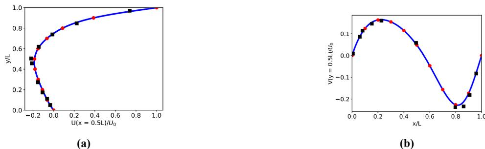
**Figure 5:** Velocity profiles from the 2D cavity case: —, cellPoint; ●, cellPointWallModified; ■, Reference data from Ghia et al. (1982)
