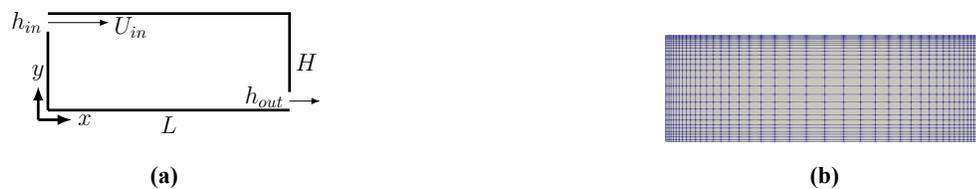
**Figure 7:** Illustration of the 2D forced convection case: (a) Schematic (based on Figure 4-9 of Zuo (2010)) (b) Mesh
