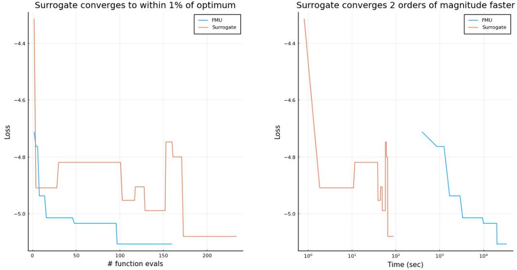
**Figure 4.** Comparison of global optimization while using the full model and the surrogate. Loss is measured using the full model’s objective function. (Left) Convergence of loss with number of function evaluations (Right) Convergence of loss with wall clock time. The optimization using the surrogate converged much before the result from the first function evaluation of the full model is over. This is why the blue line appears translated horizontally in time.
