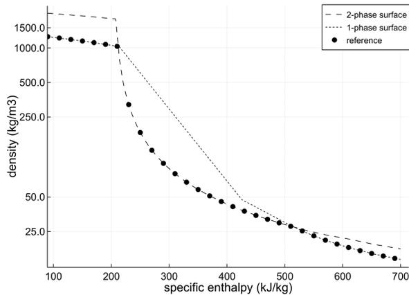
**Figure 1:** Patches  $\rho_{\varphi_1}$  and  $\rho_{\varphi_2}$  for R32 at 1 MPa compared against reference data from REFPROP.
