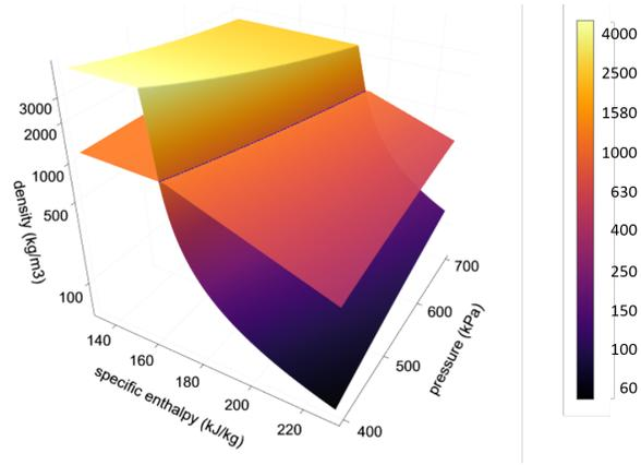
**Figure 2:** Patches  $\rho_{\varphi_1}$  and  $\rho_{\varphi_2}$  for R32 in the neighborhood of the liquid saturation curve at low pressure.
