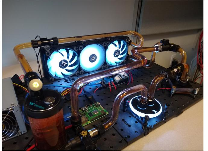
Fig. 2. Cooling Loop Test bed.
