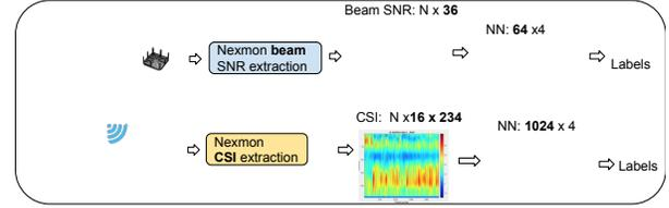
Fig. 5: Flow chart of collecting data and feeding into neural network for prediction.
