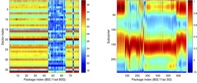
Fig. 2: The mid-grained beam SNR measurements at 60-GHz (left) and fine-grained CSI measurements at 5-GHz when a person walks through the monitoring area.
