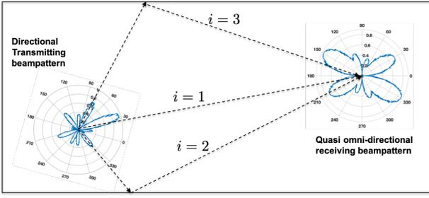
Fig. 1: Illustration of beam SNR measurements as a function of transmitting and receiving beampatterns.
