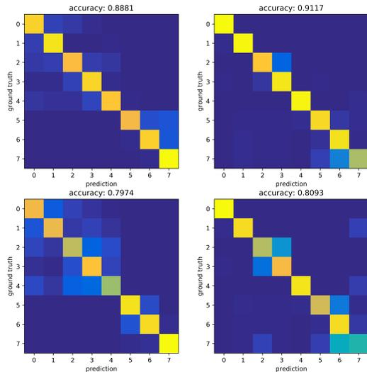
Fig. 7: Confusion matrices of Task I of human pose recognition with beam SNR (top-left) and CSI (bottom-left) and Task 2 of seat occupancy classification with beam SNR (top-right) and CSI (bottom-right). Beam SNR shows more robust performance over different sessions.
