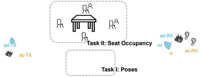
Fig. 3: Experimental setup for Task I of human pose recognition and Task II of seat occupancy sensing.
