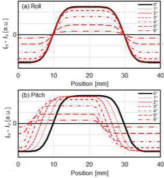
**Fig. 2.** Simulated encoder signals under (a) roll condition and (b) pitch condition. Focal length and diameter of the lens are 100 mm and 10 mm, respectively. The results under 0 and 5 degree are shown in bold for clarity.
