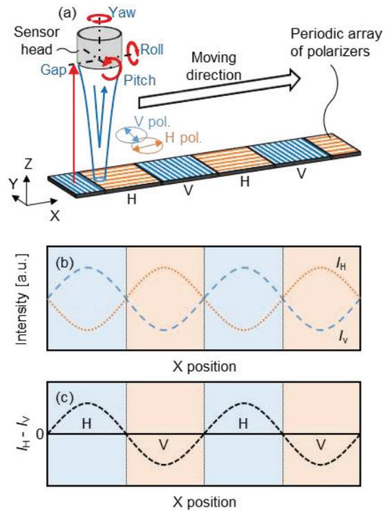
**Fig. 1.** Schematic diagram of (a) proposed THz polarimetric encoder, (b) signal traces of  $I_H$  and  $I_V$  using two orthogonally polarized beams and (c) differential signal intensity  $I_H - I_V$  using two orthogonally polarized beams.
