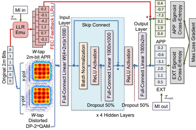
Fig. 9. DNN-TEQ architecture and min-max-loss training.
