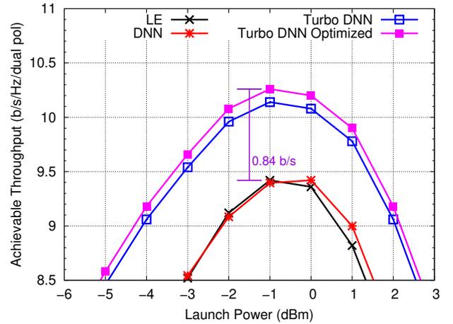
Fig. 15. Achievable rate for DP-64QAM 20-span SSMF UM links (variable-rate LDPC codes, 8-iteration BP decoding).
