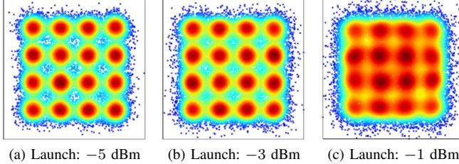
Fig. 4. Residual distortion of DP-16QAM after LE at 16-span NZDSF links.
