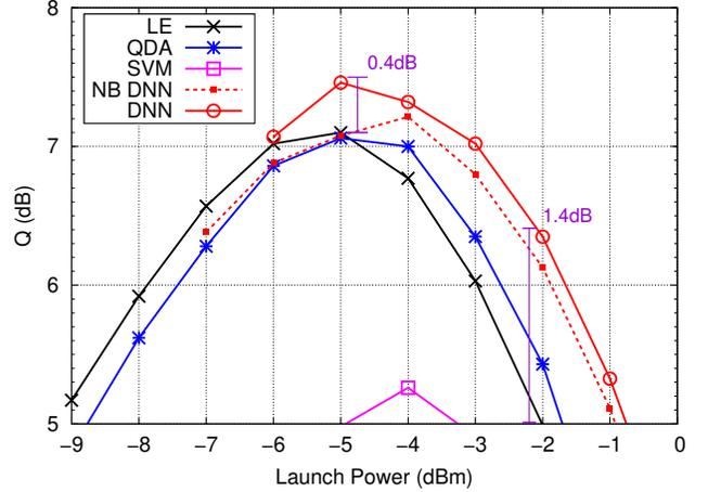
Fig. 7. Q factor comparisons for DP-16QAM 16-span NZDSF.
