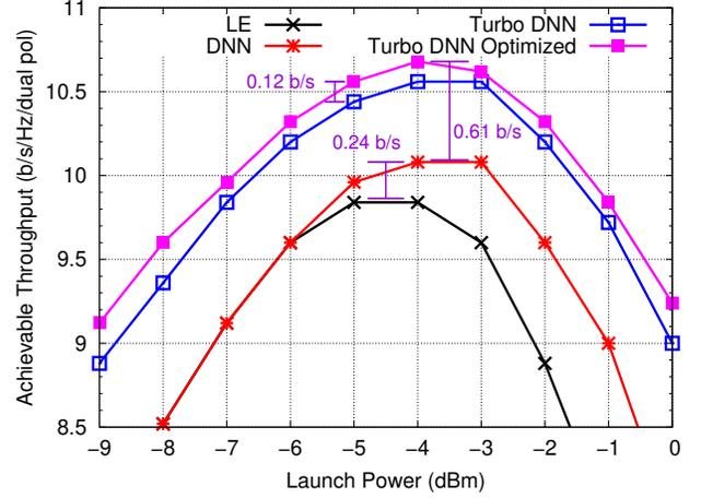
Fig. 14. Achievable rate for DP-64QAM 8-span NZDSF DM links (variable-rate LDPC codes, 8-iteration BP decoding).
