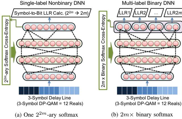
Fig. 5. Nonbinary and binary DNN equalizers for DP- $2^m$ QAM.
