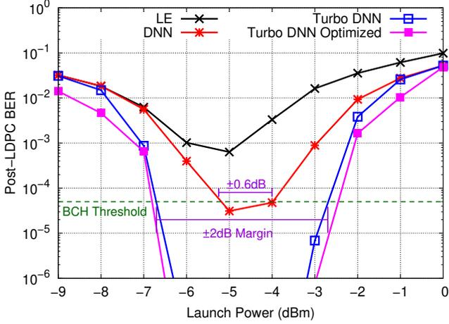
Fig. 12. BER performance for DP-16QAM 16-span NZDSF DM links (LDPC code rate 9/10, 4-iteration BP decoding).
