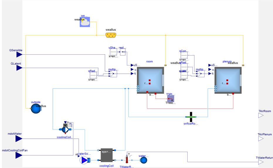
**Figure 5.** Two zone (room/plenum) model including a fan coil unit.
