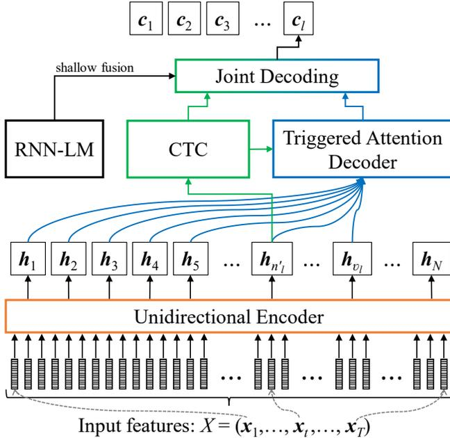
**Fig. 1.** Joint CTC-triggered attention architecture for streaming recognition.
