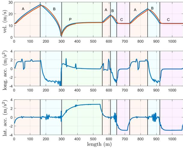
Fig. 3. Results corresponding to one lap around the track, with desired (blue) and actual (red) longitudinal velocity (top), longitudinal acceleration (middle), and lateral acceleration (bottom); transitions between maneuvers are demarcated by black vertical lines and shading and maneuvers are labeled in the top plot.
