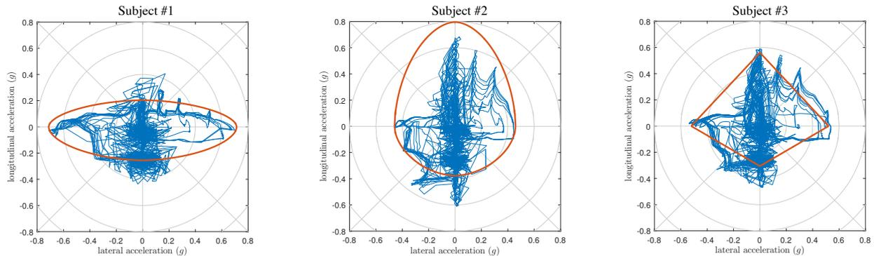
Fig. 5. Learned g-g plot (thick, red) corresponding to subjects #1-#3 with trace of acceleration applied at the vehicle's center of gravity (thin, blue).
