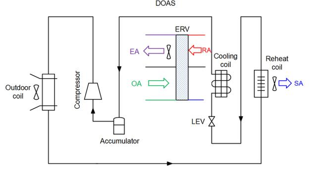
Figure 6: Construction of DOAS with reheat coil.
