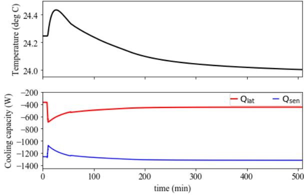
Figure 7: Ground floor zone temperature transient after 10 Hz step in compressor speed.
