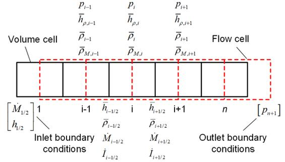
Figure 4: Finite volume discretization of refrigerant pipe.
