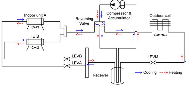
Figure 5: Construction of VRF system.
