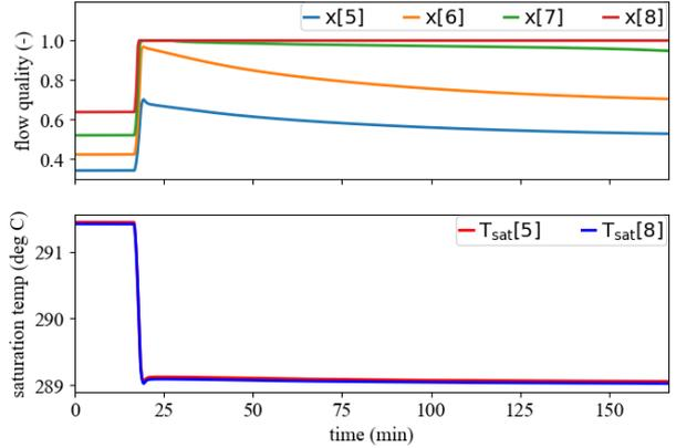
Figure 8: Flow qualities and saturation temperatures for volumes in ground floor zone heat exchanger for VRF system during compressor step transient.
