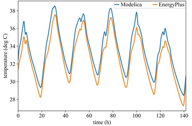
Figure 3: Comparison of ground floor convective zone temperature outputs from EnergyPlus and Modelica.
