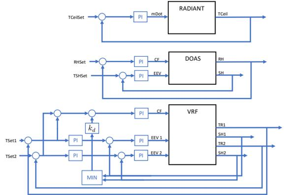
Figure 9: Feedback control architecture.
