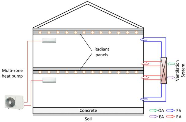
Figure 2: Overall system schematic.
