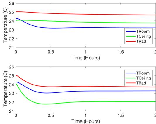
Figure 10: Temperature response of the integrated system, showing zone air temperature ( $T_{Room}$ ), ceiling panel temperature ( $T_{Ceiling}$ ), and zone mean radiant temperature ( $T_{Rad}$ ), for a  $-1\text{ }^{\circ}\text{C}$  setpoint change in air temperature (top), and a simultaneous  $-2\text{ }^{\circ}\text{C}$  setpoint change in ceiling temperature (bottom).
