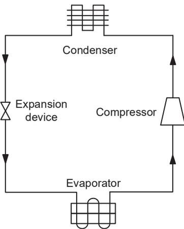
Fig. 2 Air-conditioning system
