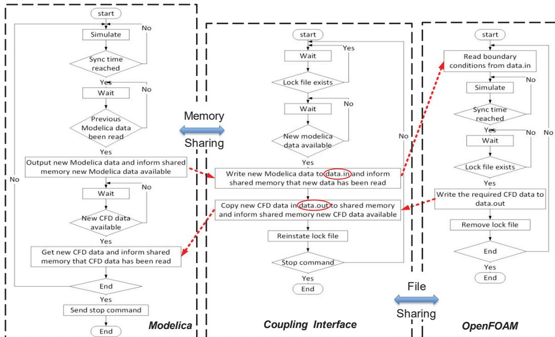
Fig. 1 Data exchange process in the coupled simulation
