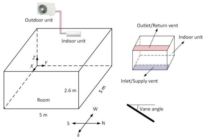
Fig. 3 CFD calculation domain
