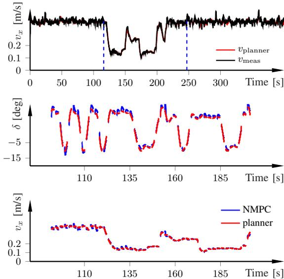
Fig. 5. Steering and velocity references (red) from the motion planner and the corresponding measured quantities throughout the experiment in the upper plot, where the portion of the data set in Fig. 4 is indicated by the blue dashed lines. The two lower plots show the steering and velocity references from the motion planner and the corresponding predicted quantities from the NMPC, at every third planning instant.
