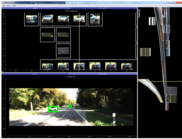
Figure 3: Zoomed-in view of Space-Time Slices (on the right) around the rectangle in Fig. 4 (c). The yellow horizontal line in the right view corresponds to the video frame shown in the bottom left view, showing that two vehicles have been detected. The top left view shows the neighboring object chains. Again the yellow line (vertical in this case) corresponds to the same frame indicated in the other views. The yellow vertical line intersects two object chains, each of which is for a detected vehicle. Other isolated image patches show false positives in nearby video frames.
