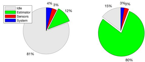
Fig. 5. CPU utilization  $\mathcal{U}$  of the Cortex M4 with  $\dim(\mathbf{y}_k) = 6$  running the EKF at  $(f_p^*, f_u^*) = (500, 100)$  [Hz] (left) and the FPF with  $N = 20$  particles and  $d\lambda = 0.1$  at  $(f_p^*, f_u^*) = (210, 100)$  Hz (right).
