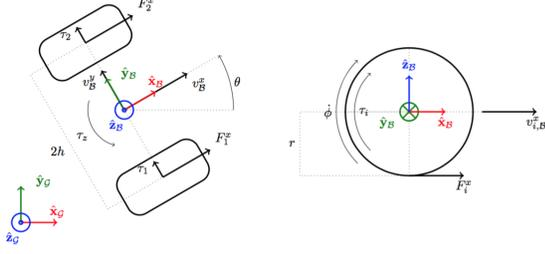
Fig. 1. Left: An  $SE(2)$  rigid-body. Right: Wheel forces.
