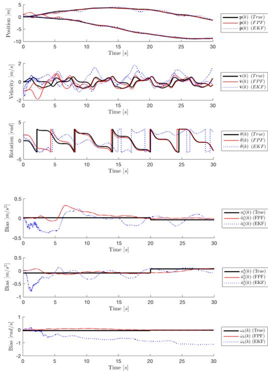
Fig. 7. True and estimated states in one of the MC-executions of problem  $\mathcal{P}_3$  using the EKF (blue) and FPF (red) with a poor initial state estimate with an added bias step change at  $t = 20$  s for demonstrative purposes.
