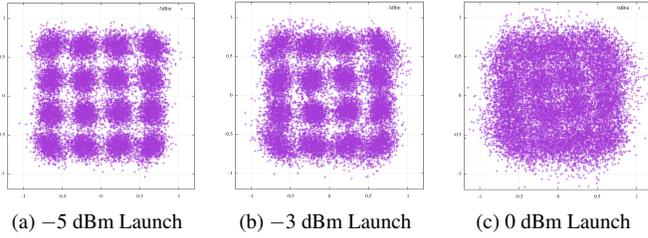
Fig. 1: Residual distortion of DP-16QAM constellation after LE for 15-span NZDSF DM links.
