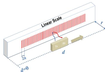
Fig. 1. The geometric configuration of linear electromagnetic encoder systems. The source transceivers are mounted on a moving read-head with a distance to the scale platform. On the scale platform, uniformly spaced bars are installed.
