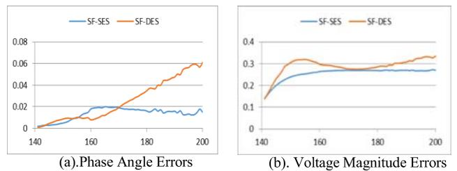
Fig. 3. MAEs of state estimations for direct state forecasting methods
