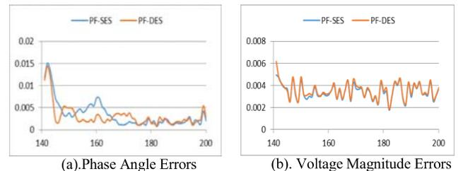
Fig. 4. MAEs of state estimations for power injection forecasting methods
