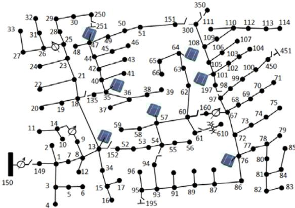
Fig. 1. A modified IEEE 123-node test feeder
