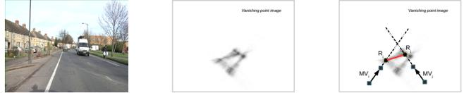
**Fig. 1.** **Left:** Example frame from a car driving sequence in [12]. **Center:** Motion vanishing point image for that frame. **Right:** Representation point of a MV and perspective distance between a pair of MVs.
