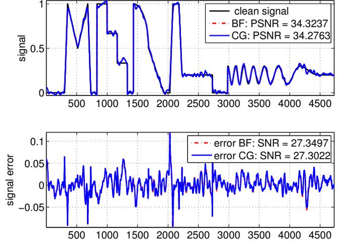
Fig. 2. 500 BF iterations versus 20 CG-BF iterations with the guidance  $x_c$ .
