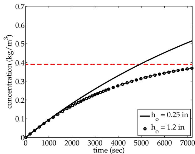
Figure 6:  $\bar{C}$  over 7200 seconds during a low-rate leak for cases where  $h_{out}$  varies between 0.25 and 1.2 inches, with  $Q_{exh} = 5$  cfm. The RCL is denoted by the dashed line.
