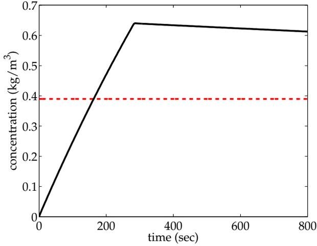
Figure 1:  $\bar{C}$  during a high-rate leak, with a  $Q_{exh} = 5$  cfm and  $h_{out} = 0.25$  in, over 800 seconds. The RCL is denoted by the dashed line.
