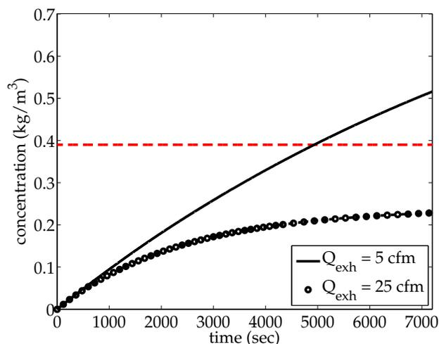
Figure 8:  $\bar{C}$  over 7200 seconds during a low-rate leak for cases where  $h_{out}$  varies between 0.25 and 1.2 inches, with  $Q_{exh} = 5$  cfm. The RCL is denoted by the dashed line.
