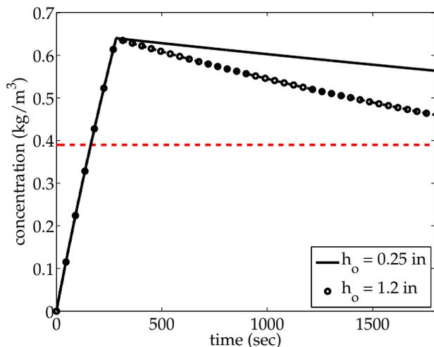
Figure 5:  $\bar{C}$  over 1800 seconds during a high-rate leak for cases where  $h_{out}$  varies between 0.25 inches and 1.2 inches, with  $Q_{exh} = 5$  cfm. The RCL is denoted by the dashed line.
