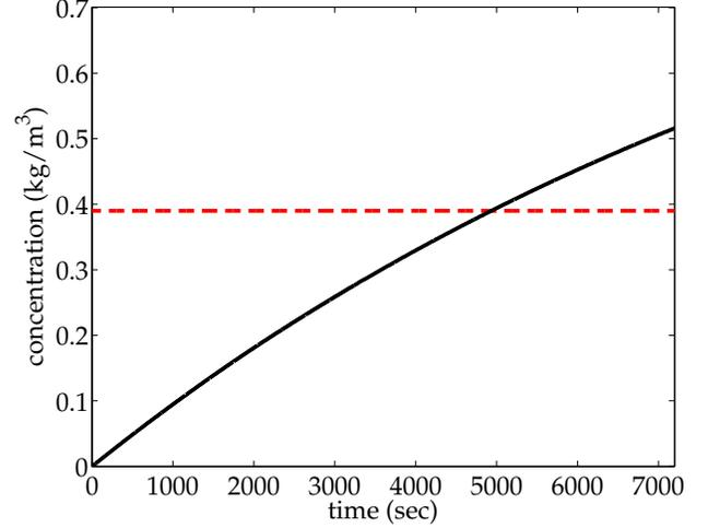
Figure 2:  $\bar{C}$  during a low-rate leak, with  $Q_{exh} = 5$  cfm and  $h_{out} = 0.25$  in, over 7200 seconds. The RCL is denoted by the dashed line.
