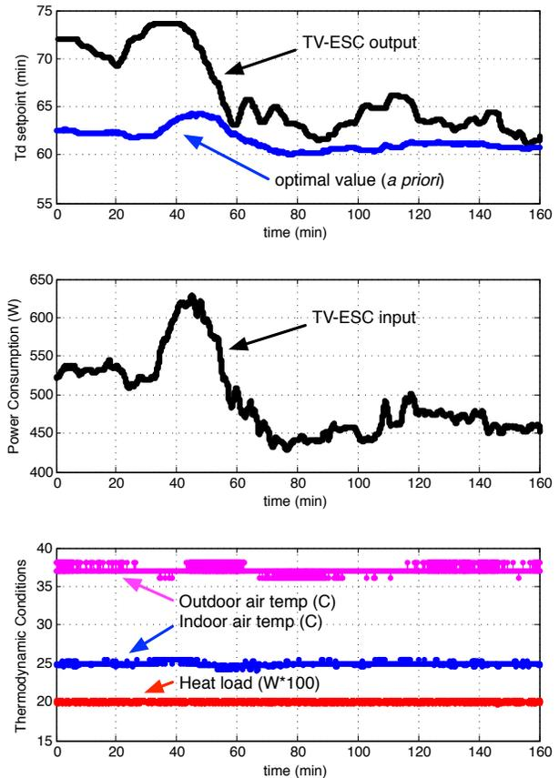
Fig. 4. Top: The discharge temperature setpoint (black) is driven to the optimal setpoint (blue) determined from previous experiments in about  $160 \text{ min}$ . Middle: The power consumption for this test is driven from an initial value of about  $525 \text{ W}$  to about  $450 \text{ W}$  while the thermodynamic conditions are held constant (bottom).
