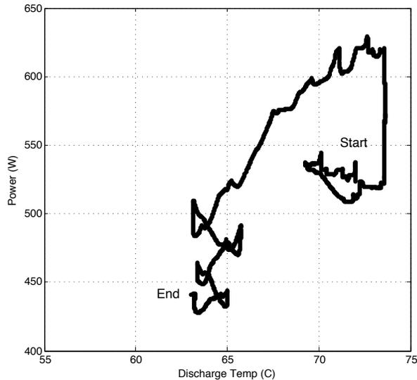
Fig. 5. Power consumption optimization for the room air conditioner.
