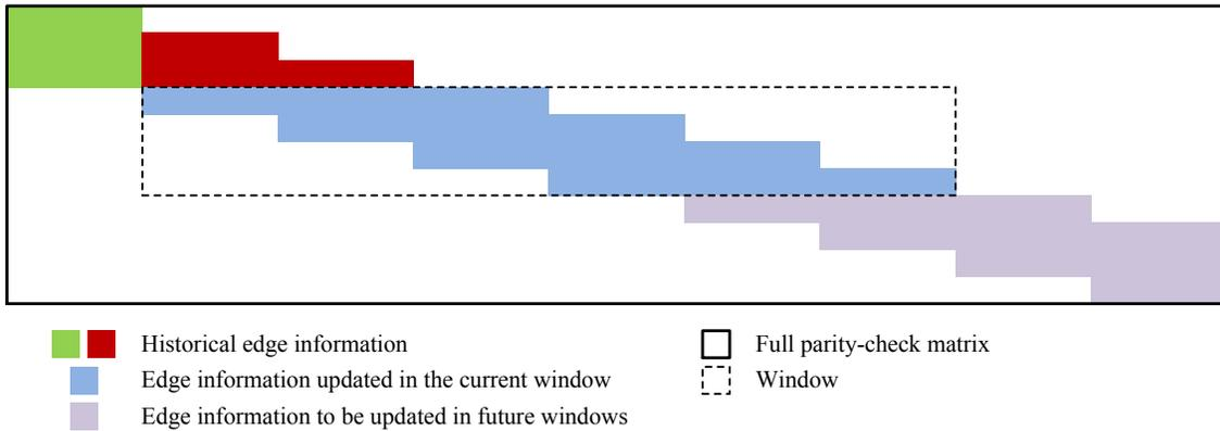
Fig. 1.  $(3, 15, 9, M)$  LDPC-CC's PCM and window decoding with window size  $W = 4$  at the 4-th decoding instant.
