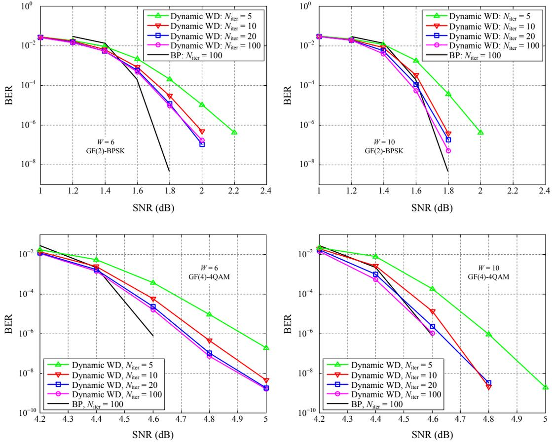
Fig. 2. The BER performances of dynamic WD scheme with window size  $W = 6, 10$  for  $N_{\text{iter}} = 5, 10, 20, 100$ .
