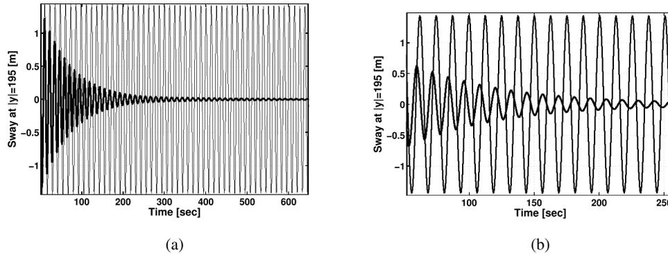
Fig. 2. Rope sway at  $y = 195$  m in the case of nonzero initial conditions and zero external disturbance. (a) Rope sway at  $y = 195$  m: no control (thin line) and with control (12) (bold line). (b) Zoom of the rope sway at  $y = 195$  m: no control (thin line) and with control (12) (bold line).
