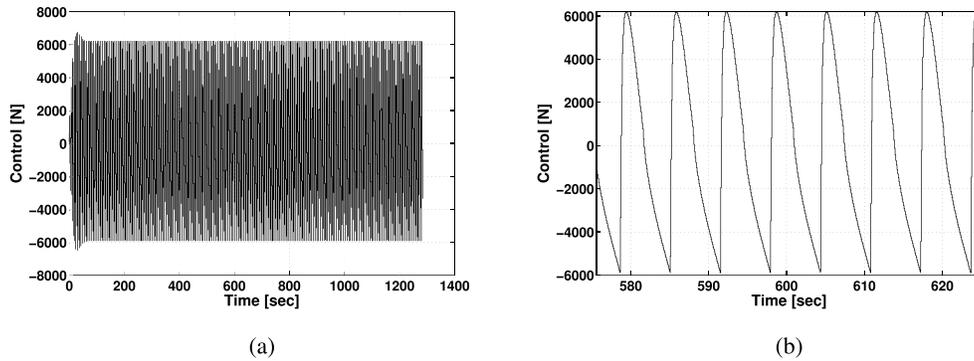
Fig. 10. Output of controller (25) in the case of nonzero external disturbance and time-varying rope length. (a) Output of controller (25). (b) Output of controller (25) zoomed-in view.
