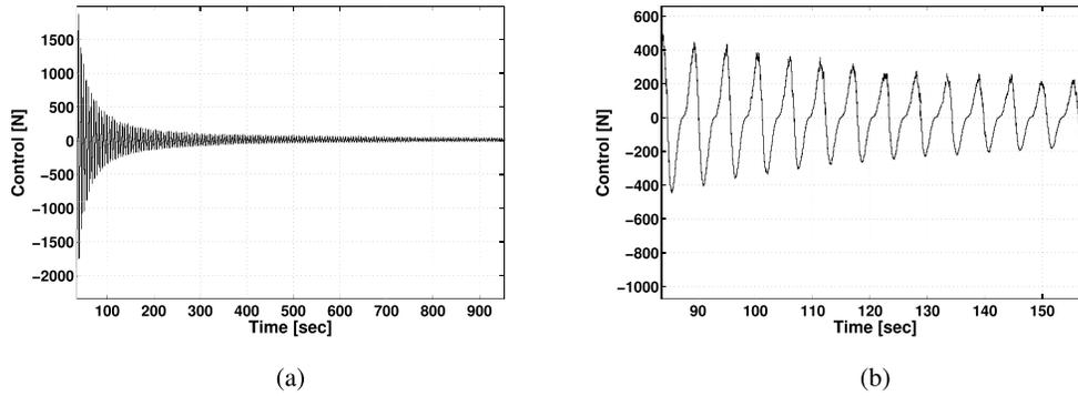
Fig. 8. Output of controller (18) in the case of nonzero initial conditions, without external disturbance and time-varying rope length. (a) Output of controller (18). (b) Output of controller (18) zoomed-in view.
