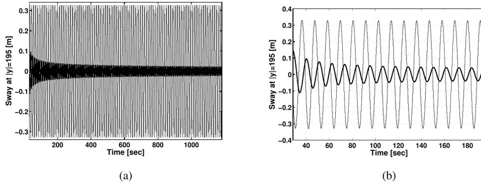
Fig. 7. Rope sway at  $y = 195$  m in the case of nonzero initial conditions, without external disturbance and time-varying rope length. (a) Rope sway at  $y = 195$  m: no control (thin line) and with control (18) (bold line). (b) Zoomed-in-view of rope sway at  $y = 195$  m: no control (thin line) and with control (18) (bold line).
