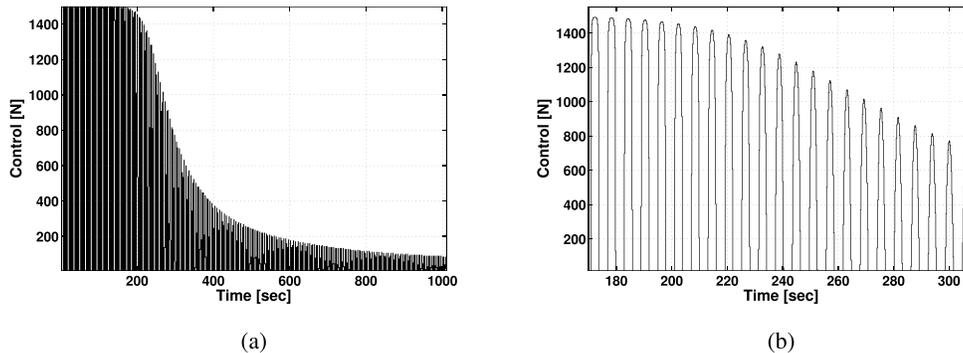
Fig. 3. Output of controller (12) in the case of nonzero initial conditions and zero external disturbance. (a) Output of controller (12). (b) Output of controller (12) zoomed-in view.
