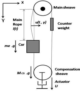
Fig. 1. Schematic representation of an elevator shaft showing different variables used in the model.
