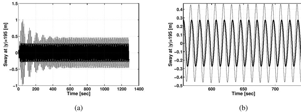
Fig. 9. Rope sway at  $y = 195$  m with external disturbance and time-varying rope length: no control (thin line) and with control (bold line). (a) Rope sway at  $y = 195$  m: no control (thin line) and with control (25) (bold line). (b) Zoomed-in-view of rope sway at  $y = 195$  m: no control (thin line) and with control (25) (bold line).
