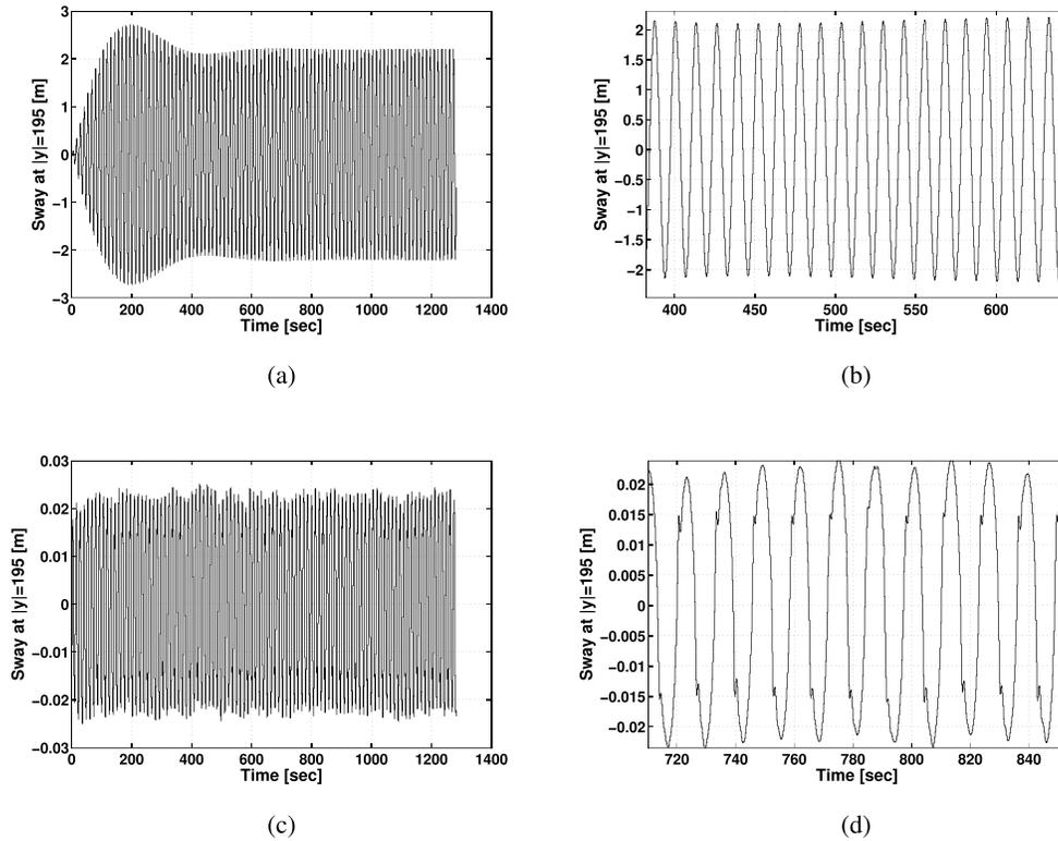
Fig. 4. Rope sway at  $y = 195\text{ m}$  in the case of nonzero external disturbance. (a) Rope sway at  $y = 195\text{ m}$  without control. (b) Zoomed-in-view of rope sway at  $y = 195\text{ m}$  without control. (c) Rope sway at  $y = 195\text{ m}$  with control (15). (d) Zoomed-in view of the rope sway at  $y = 195\text{ m}$  with control (15).
