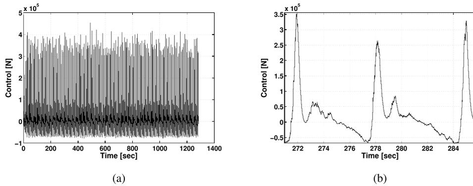
Fig. 5. Output of controller (15) in the case of nonzero external disturbance. (a) Output of controller (15). (b) Output of controller (15) zoomed-in view.
