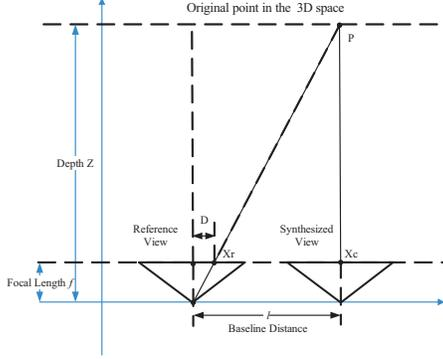
**Fig. 2.** Depth-assisted image rendering
