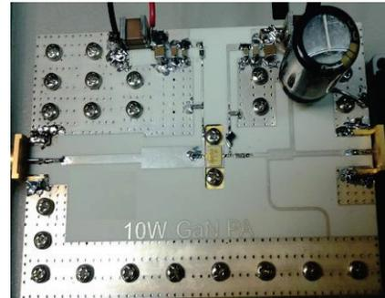
Fig. 5. Fabricated 10W high voltage GaN power amplifier.
