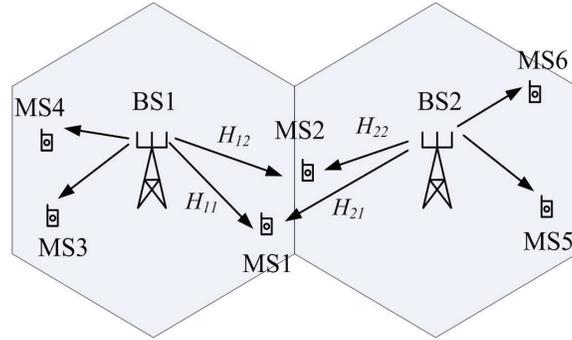
Fig. 3. Model of CoMP Joint Transmission
