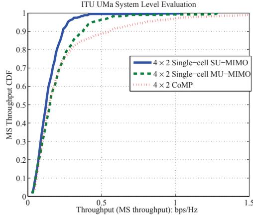
Fig. 4. System Performance Comparison
