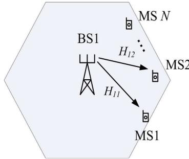
Fig. 2. Model of Single-Cell MU-MIMO System
