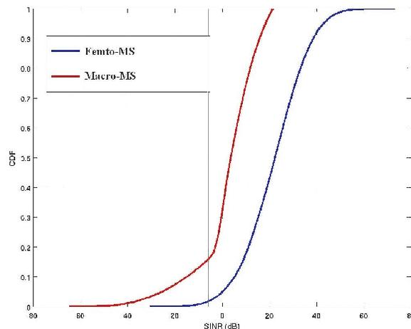
Fig. 6. MMS and FMS SINR without power setting
