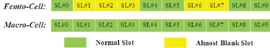
Fig. 7. Time-domain solution for inter-cell interference coordination
