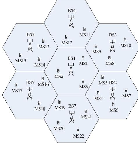
Fig. 1. Model of a Multi-Cell System
