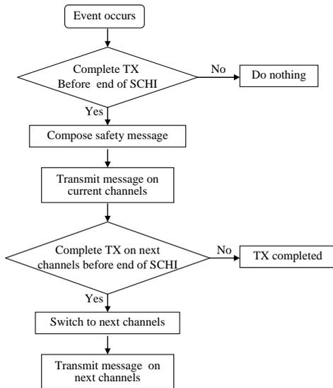
Figure 5. Source Vehicle Safety Message Transmission in SCHI
