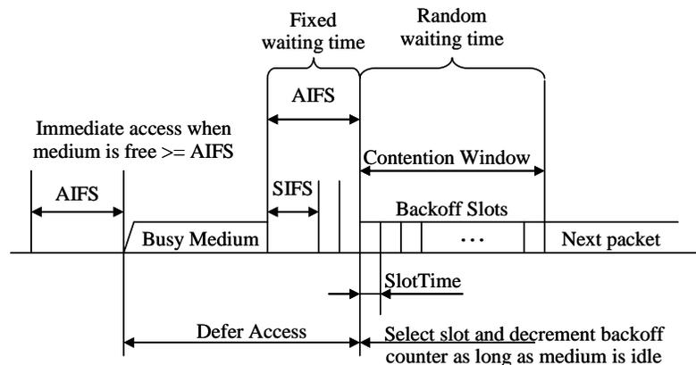
**Figure 8. EDCA Channel Access Illustration**
