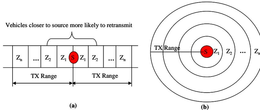
**Figure 7. Safety Message Retransmission Zone Partitioning**
