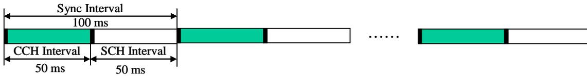
Figure 2. WAVE Sync Interval Partitioning
