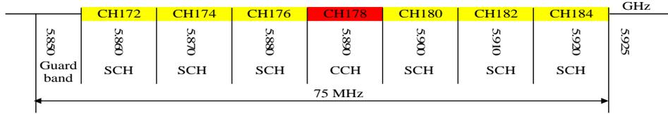
Figure 1. Frequency Channel Layout of 5.9 GHz Band
