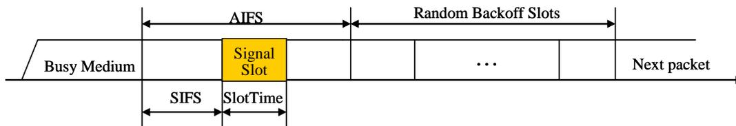
**Figure 9. Signal Slot Selection**
