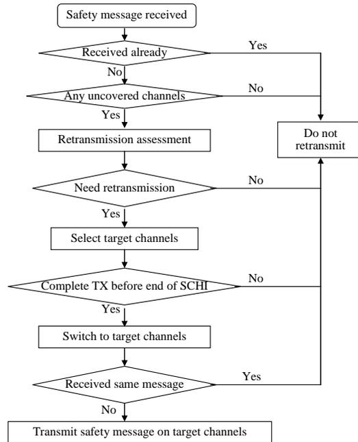
Figure 5. Source Vehicle Safety Message Transmission in SCHI Figure 6. Neighbor Vehicle Safety Message Relay in SCHI
