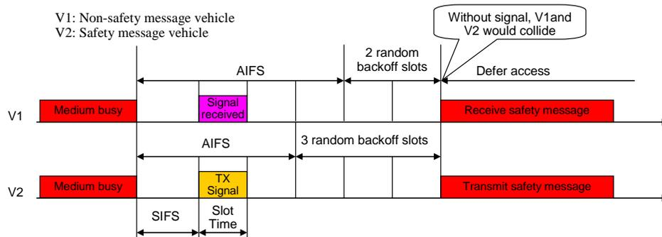
Figure 11. Example of Signalling Avoiding Collision
