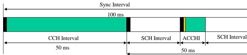
Figure 14. WAVE Sync Interval with one ACCHI Inserted in SCHI
