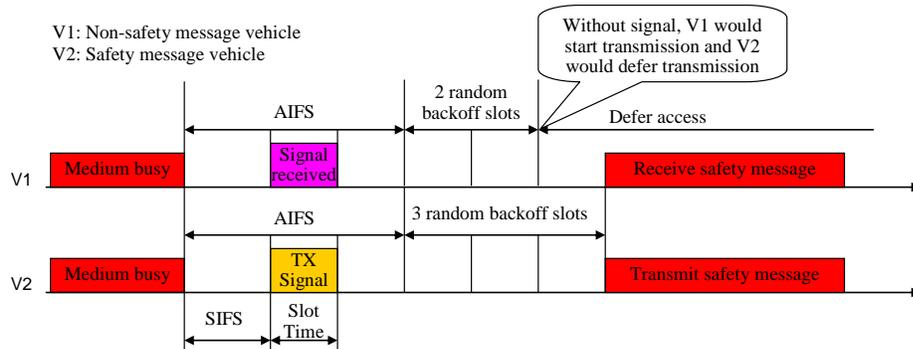
Figure 10. Example of Signalling for Safety Message Transmission
