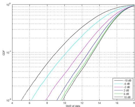
Fig. 5. Entire bandwidth assigned to 25 MSs ( $f_d = 5$  Hz, frequency-domain scheduling, sounding RS sent every 2 TTI)
