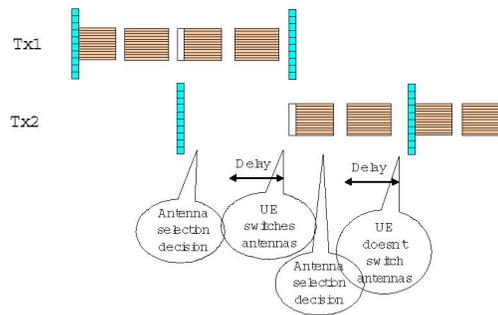
Fig. 1. Uplink transmit antenna selection training using sounding reference signals
