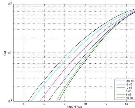
Fig. 2. Entire bandwidth assigned to 25 MSs ( $f_d = 5$  Hz, round-robin scheduling, sounding RS sent every TTI)
