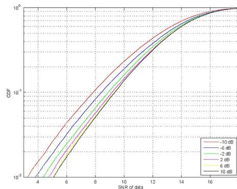
Fig. 3. Entire bandwidth assigned to 5 MSs ( $f_d = 10$  Hz, round-robin scheduling, sounding RS sent every 2 TTI)
