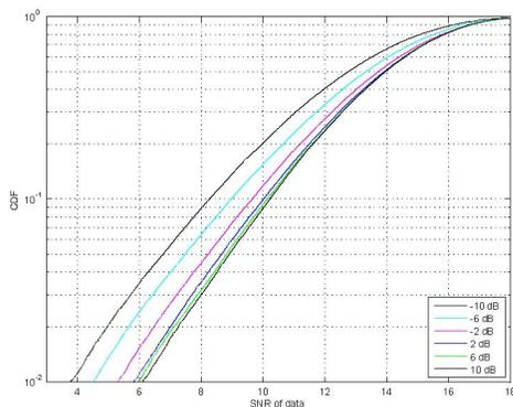
Fig. 6. Entire bandwidth assigned to 5 MSs ( $f_d = 10$  Hz, frequency-domain scheduling, sounding RS sent every 2 TTI)
