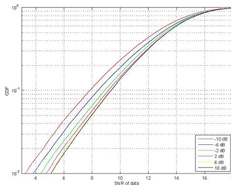
Fig. 3. Entire bandwidth assigned to 5 MSs ( $f_d = 10$  Hz, round-robin scheduling, sounding RS sent every 2 TTI)
