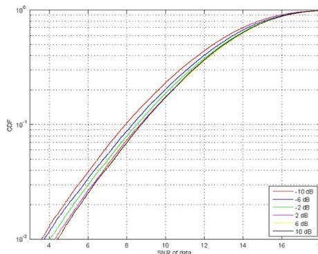
Fig. 4. Entire bandwidth assigned to 2 MSs ( $f_d = 10$  Hz, round-robin scheduling, sounding RS sent every 2 TTI)
